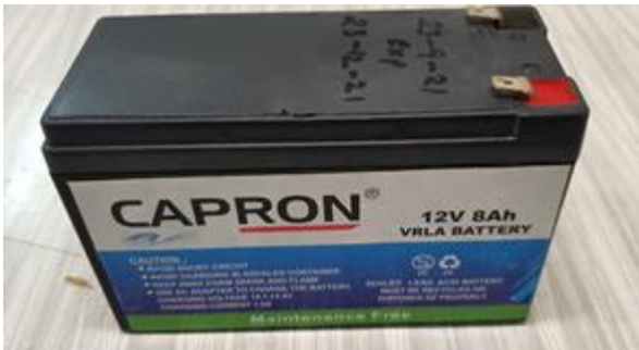
Figure 12 : Lead Acid Battery
